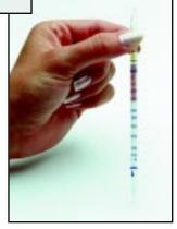
Whether in the laboratory or out at the job-site, obtain accurate ion specific measurement of chlorides from 0 - 2,000 ppm. Use CHLOR\*TEST "W" for water and many other liquids.
