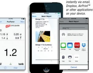
PosiTector SmartLink accepts PosiTector 6000, SPG, RTR-H, and DPM probes easily converting to a coating thickness gage, surface profile gage or dew point meter.
