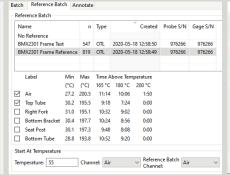
**Reference Batch**—store optimal cure reference profiles to compare measurement results
