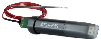
This standalone data logger measures and stores more than 32,000 temperature readings from a J, K or T-type thermocouple at a resolution of 0.5°C (1°F). It comes supplied with a K-type thermocouple capable of measuring from 0 to +200°C (+32 to +392°F).
