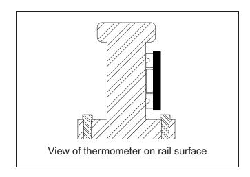
PTC® Industrial Railroad Thermometers conform to AREMA Specifications and are engineered to measure surface temperatures. Four alinico magnets form a base providing increased holding power.
