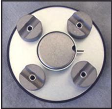
Railroad surface thermometers feature a serialized dial, protective cap for the bimetal sensor, and a powerful 4-magnet base
