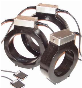
Western's new WA-Series of AC Coils are the most powerful Portable AC Coils in the inspection World. All 4 models are rated at over 4000 Amp Turns at 115VAC / 60Hz, and in excess of 5000 Amp Turns at 230VAC / 50Hz ("K" Models). The new WA-Series Coils have ID sizes that correspond to the model number; WA-8, WA-10, WA-12, and WA-14, with diameters of 203mm (8"), 254 (10"), 305mm (12"), and 356mm (14"). These 4 new models replaced our dated WAC-10.
